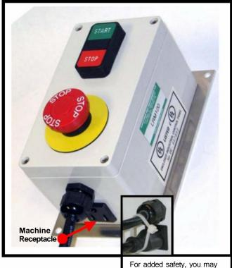
For added safety, you may use a non-conductive wire tie to bundle the 13370 cord to the machine's cord
