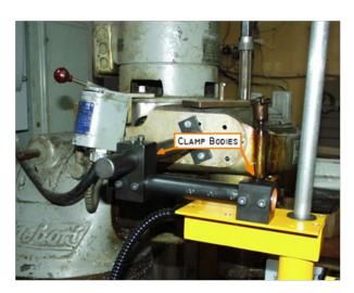
Slide the clamp bodies over the bars and tighten the hex clamping screws. You will need to readjust the X, Y and Z adjustments to position the shield properly. The trick here is to leave one of the two clamp screws loose while you position. After final position is established, tighten all screws in the clamp bodies.
