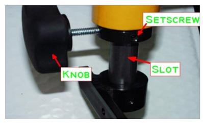
Tighten the large black height adjustment knob so the vertical post is approximately at half mast.
