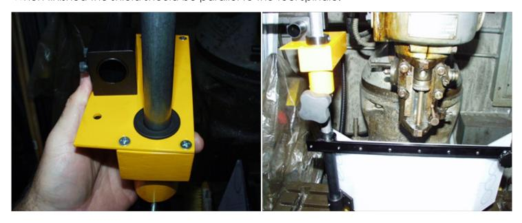
When the shield is parallel, the switch in the interlock is made/ Normally Closed.
