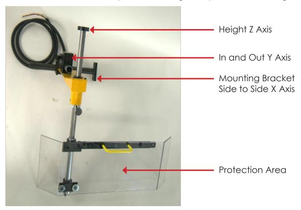
First visualize the unit mounted on your machine with the protection area centered over your tool region. The guarding system's three axis of adjustment will have to be positioned accordingly.
