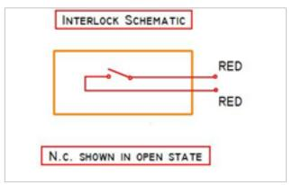
Safety Guard should be wired in series with the stop circuit of your machine.
